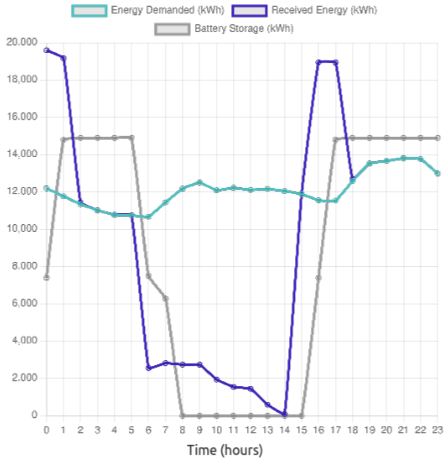
Fig. 6. Energy received by a holon representing region in the island, in a scenario where it is disconnected from the grid and the only energy and storage available are the energy produced and the storage available locally in the region.
