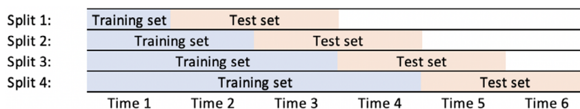
Figure 7. Illustration of the idea of walk forward validation on time-series data with sliding window.
