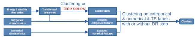
Figure 3: Clustering on mixed features and pre-clustered Time Series labels as categorical features.
